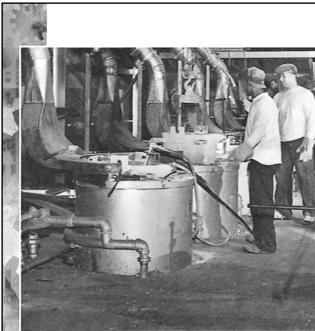
Figure 18-9. The fumes arising from lead-melting operations are controlled by local lateral-slot exhaust ventilation. (Courtesy Ford Motor Co.)
