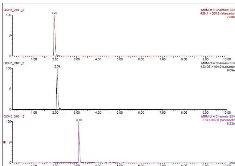
**Fig. 3: Chromatogram of irbesartan, sinensetin and losartan simultaneously**
