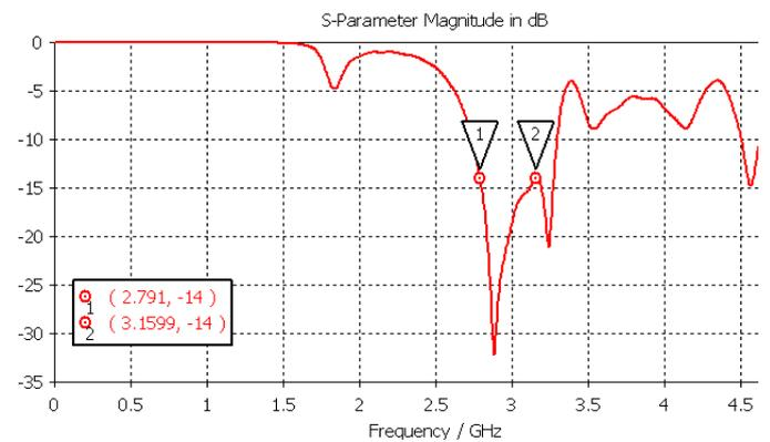
Figure 5. Simulation result of proposed modified horn antenna
