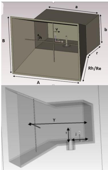
Figure 2. Parameters of the modified horn antenna
