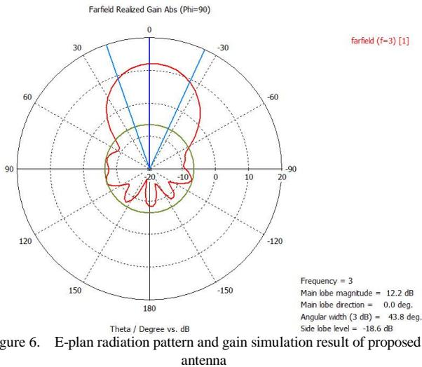
Figure 6. E-plan radiation pattern and gain simulation result of proposed antenna
