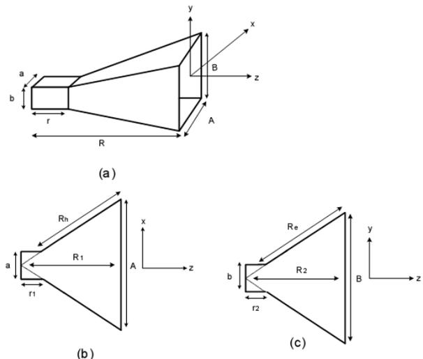
Figure 1. Parameters of conventional pyramidal horn antenna (a) 3D view (b) xz view (c) yz view [1]
