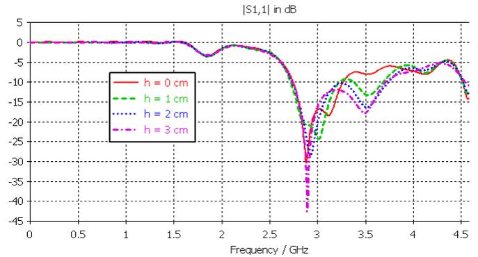
Figure 4. Influence of the metal rod in the horizontal plane towards  $S_{11}$  parameter
