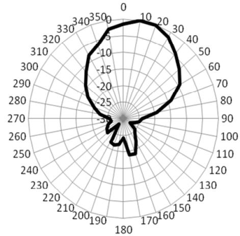
Figure 8. E-plan radiation pattern and gain simulation result of proposed antenna
