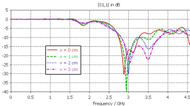
Figure 3. Influence of the metal rod in the vertical plane towards  $S_{11}$  parameter
