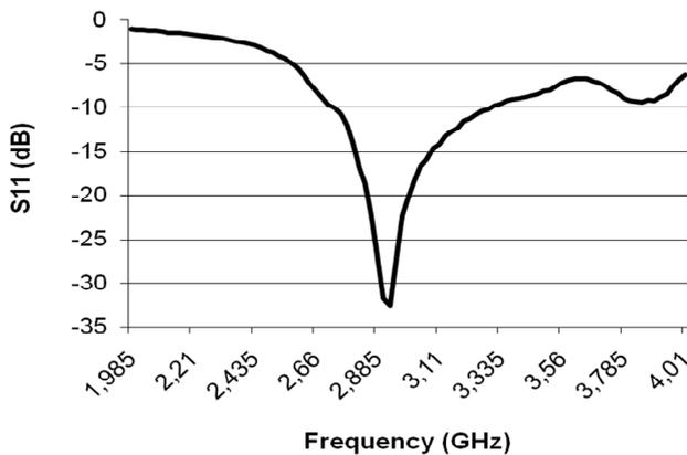
Figure 7. Simulation result of proposed modified horn antenna
