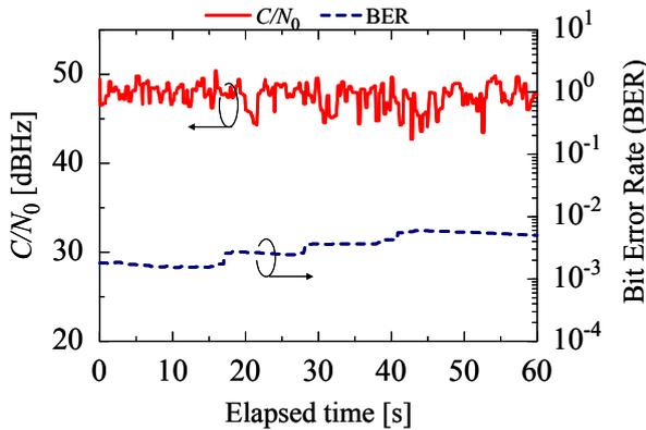
Figure 6. Carrier to noise density and BER performance in sparse foliage environment.
