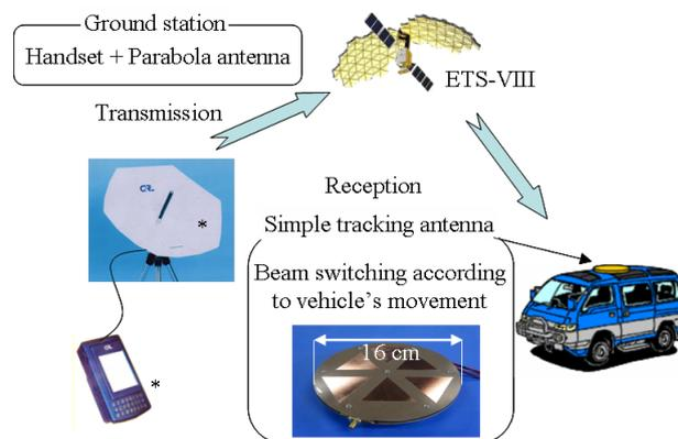
Figure 1. Experimental structure for antenna system measurement using the geostationary satellite. (\* NICT Japan)
