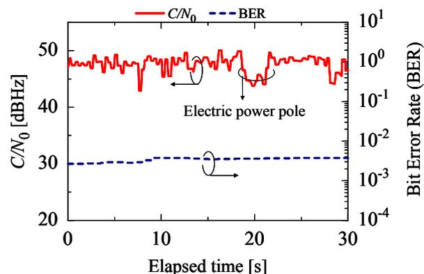
Figure 5. Carrier to noise density and BER performance when signal is blocked by a single pole.
