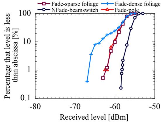
Figure 8. Fade percentage distribution due to vegetation and pole compared with the non-fade signal.
