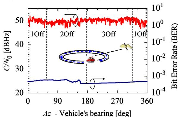
Figure 3. Carrier to noise density and BER performance for automatic satellite-tracking when vehicle turning round in circular path at LOS area.
