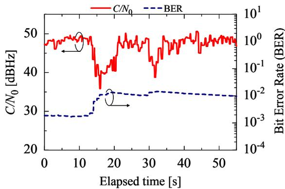
Figure 7. Carrier to noise density and BER performance in dense foliage environment.
