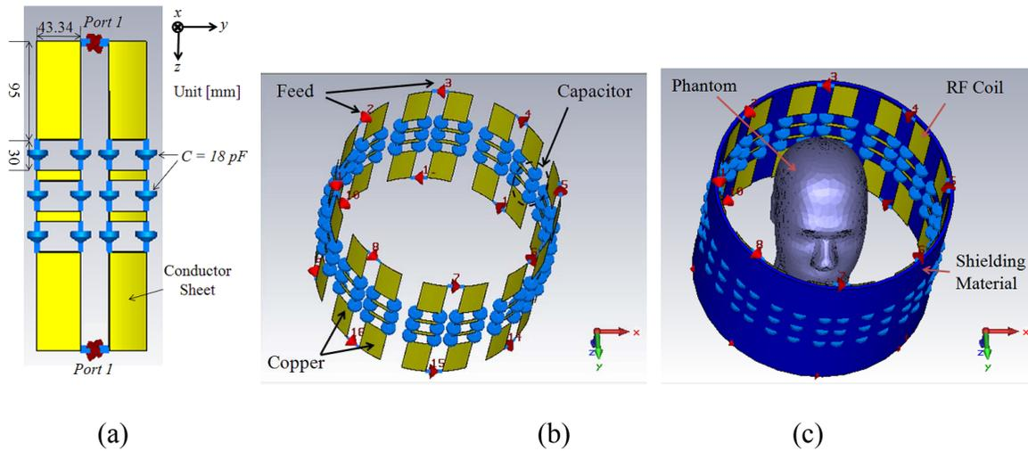
Figure 1. RF array coil structure (a) one element coil (b) 8-element array (c) array with dielectric shielding and head phantom
