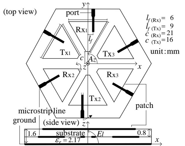
Fig. 6. Dual-band triangular-patch array antenna with truncated tip
