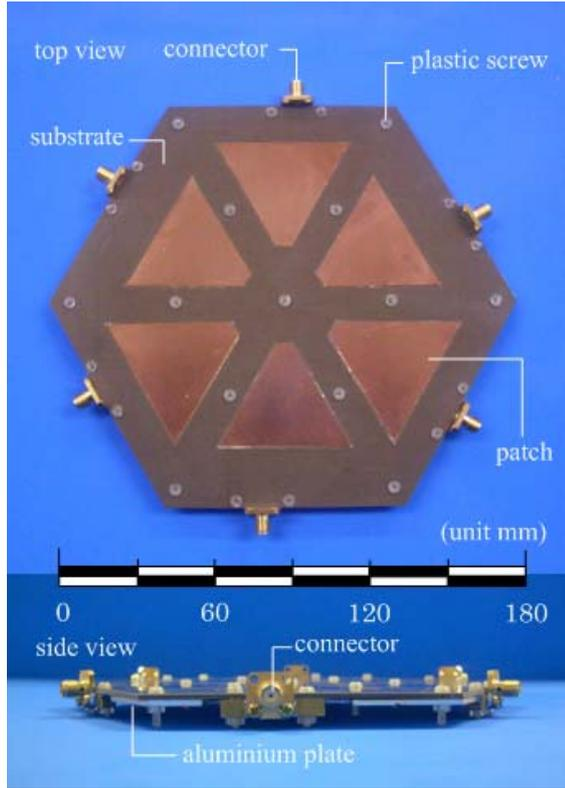
Fig. 7. Fabricated antenna
