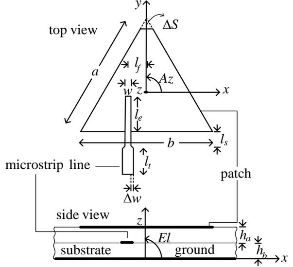
Fig. 2. Configuration of single patch antenna
