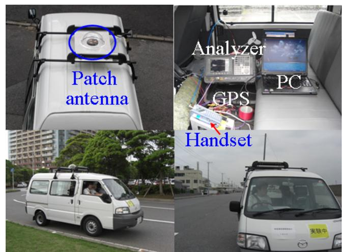
Fig.5 Photograph of outdoor measurement circumstance
