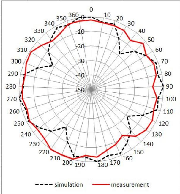
Fig. 5. Radiation pattern comparison between simulation and experiment result at  $\phi = 0$ .
