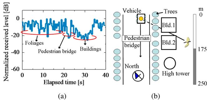
Fig. 8. Received power level in urban area (a) measurement result (b) measurement circumstance
