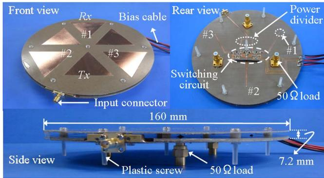
Fig. 3. Dual-band operation fabricated patch array antenna which used during field experiment.
