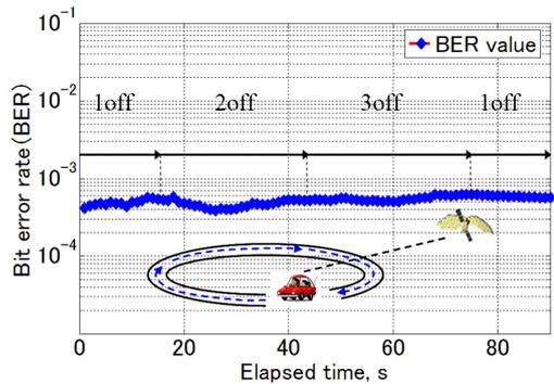
Fig. 7. Measured bit error rate (BER) of satellite-tracking when the vehicle moved at the rotary.
