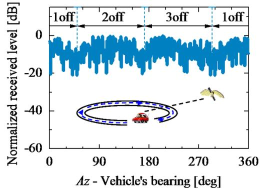
Fig. 6. Received power levels of satellite-tracking when the vehicle moved at the rotary.
