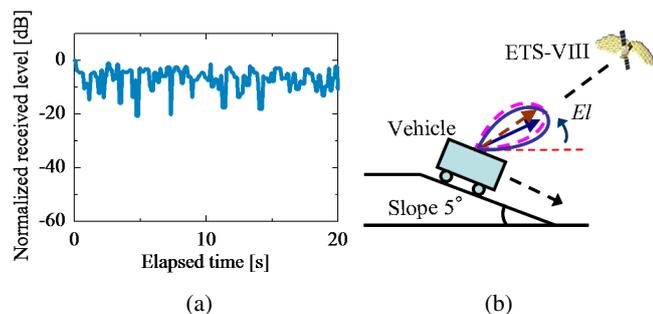
Fig. 9. Received power level in inclined-road (a) measurement result (b) measurement circumstance
