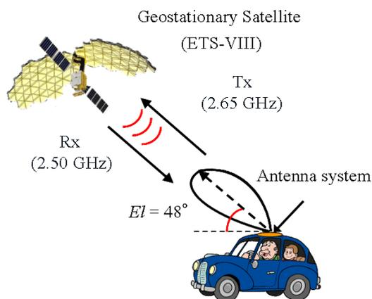
Fig. 1. Concept of antenna system aimed at vehicle communications using the satellite.
