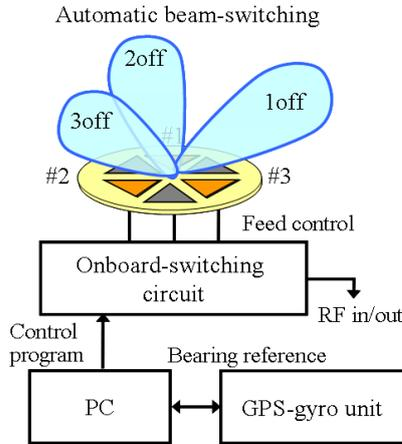
Fig. 2. Antenna system architecture which is mounted in a vehicle aimed at field experiment.
