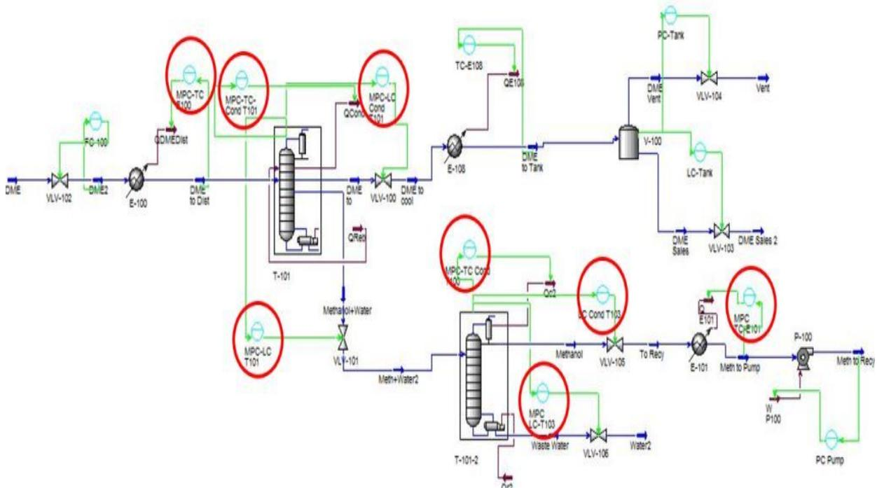
FIGURE 1. Unisim model of purification DME process
