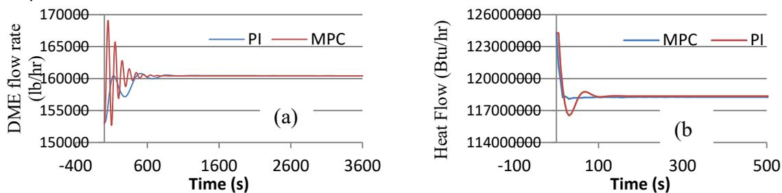
FIGURE 3. Product flow rate and utility due to changes in disturbance by 5%
