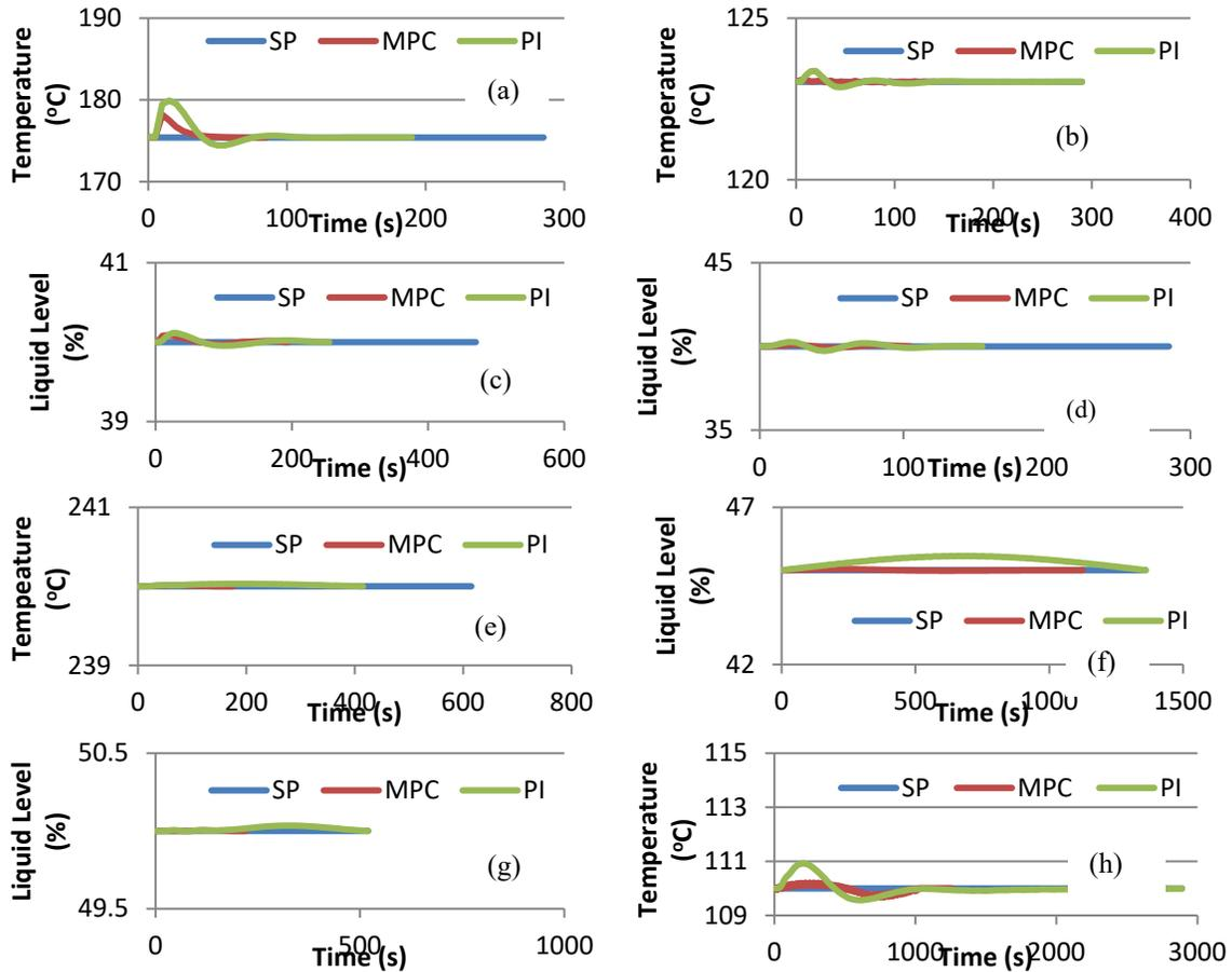
**FIGURE 2.** Control performance cause of disturbance change of 5% on feed flow rate
