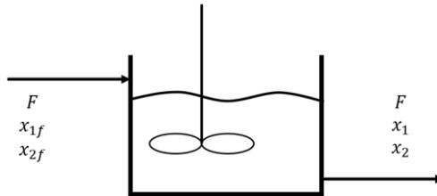
**FIGURE 1.** Biochemical reactor simplified process flow diagram
