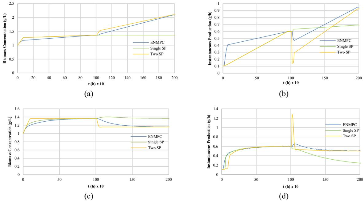
**FIGURE 2.** Controlled system dynamic concentration profile to +50% (a) and -14% (c) disturbance of  $x_{2f}$  and their respective instantaneous production dynamic profile (b,d) for monod kinetics
