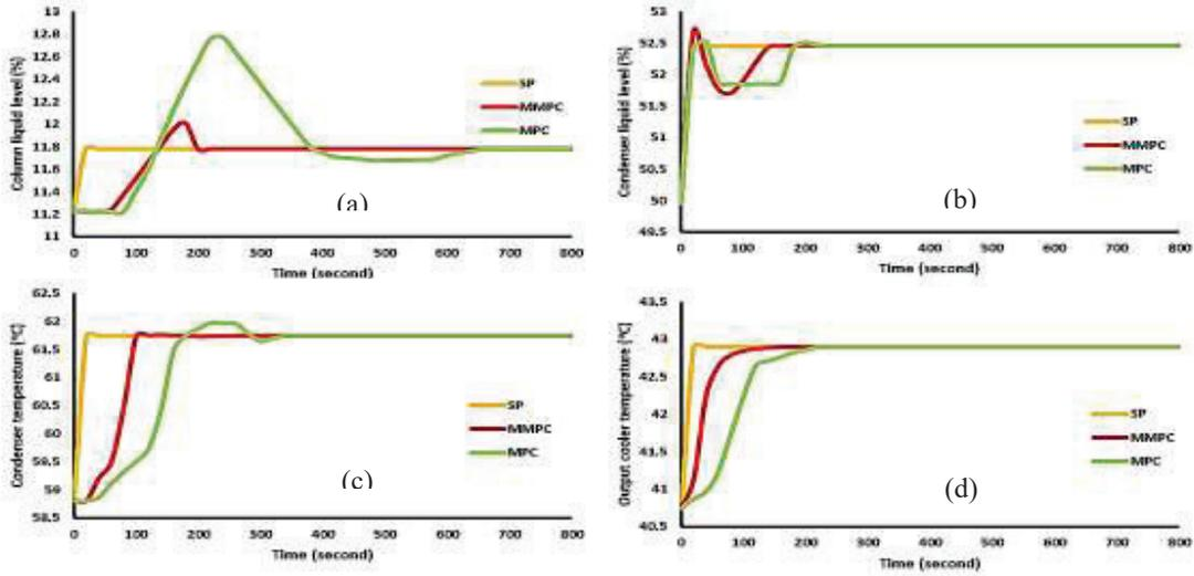
FIGURE 2. Response of control against SP changes in variable (a) column level; (b) condenser level; (c) condenser temperature; (d) temperature output cooler.
