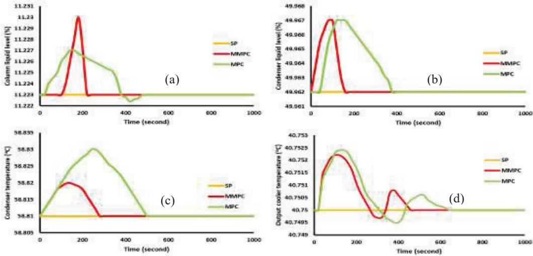
FIGURE 3. Response of control against disturbances in variable (a) column level; (b) condenser level; (c) condenser temperature; (d) temperature output cooler.
