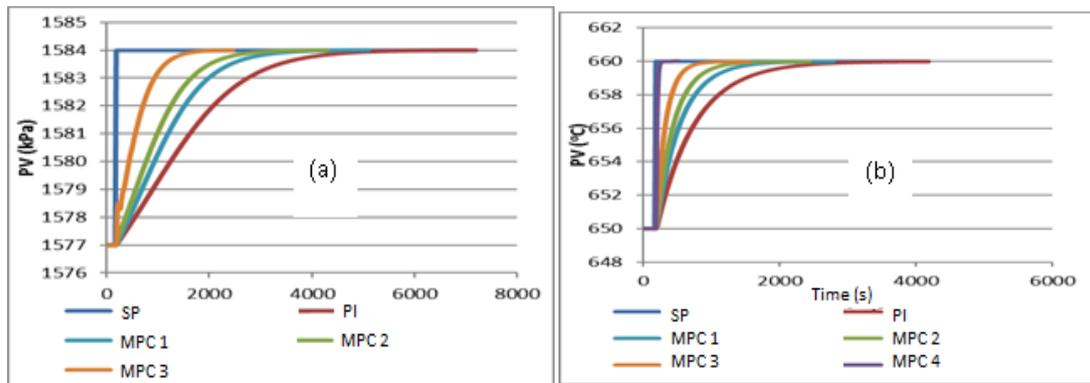
**Figure 3** PRC of (a) Pressure Control in compressor, (b) Temperature Control of heater unit in Steam Reformer
