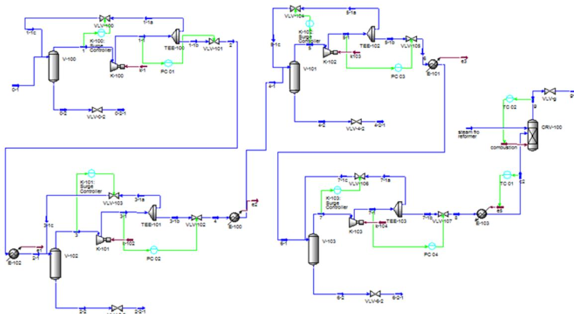
**Figure 2** Compressor and steam reformer controls using UniSim<sup>(R)</sup>
