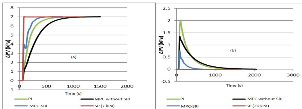
**Figure 4** PV Responses of MPC and PI in Compressor Unit-3 at (a) setpoint of +7 kPa and (b) disturbance in inlet pressure of 20 kPa
