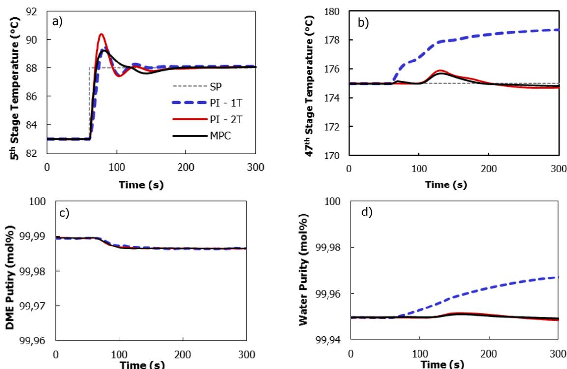
**Figure 5.** Dynamic responses to a change in stage 5 temperature set-point: a) stage 5 temperature, b) stage 47 temperature, c) DME purity, d) water purity.
