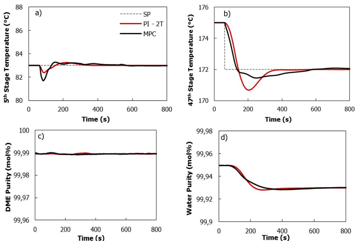
**Figure 6.** Dynamic responses for to a change in stage 47 temperature set-point: a) stage 5 temperature, b) stage 47 temperature, c) DME purity, d) water purity.
