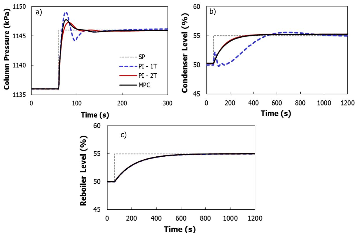
**Figure 7.** Dynamic responses to a change in the set-point of a) top column pressure, b) condenser accumulator level, c) reboiler level.
