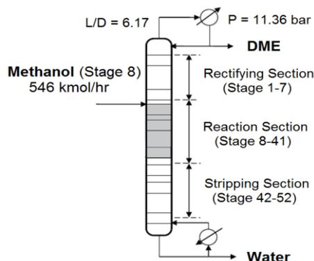
**Figure 1.** Schematic diagram of reactive distillation for the base case steady-state condition.
