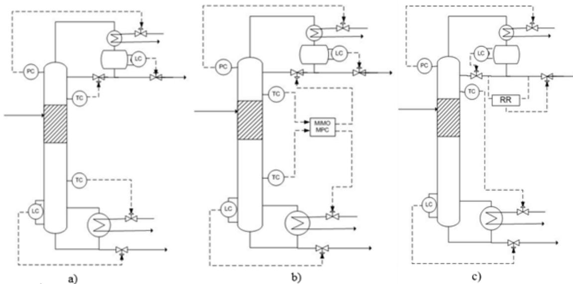
**Figure 4.** a) Two-point PI control configuration, b) MPC control configuration, c) Single-point PI control configuration.
