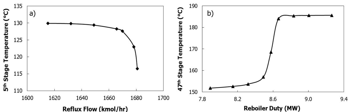
Figure 3. Steady-state input-output relation of a) reflux flow rate to stage 5 temperature, b) reboiler duty to stage 47 temperature.
