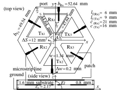
Fig. 1. Dual-band configuration of patch array antenna
