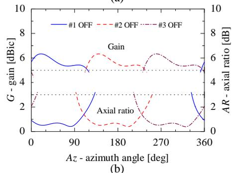
Fig. 3. Gain and axial ratio in the conical-cut plane at elevation angle El = 48° (a) Reception (b) Transmission
