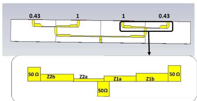
Fig 2. Unequal 4-way power divider
