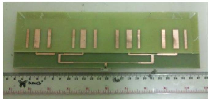
Fig 6. Photo of the fabricated antenna
