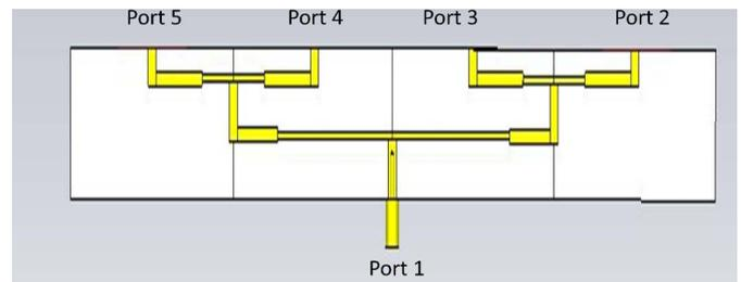
Fig 1. Equal 4-way power divider
