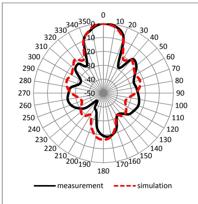
Fig 5. Radiation pattern of the antenna with unequal power divider at  $\phi = 0$
