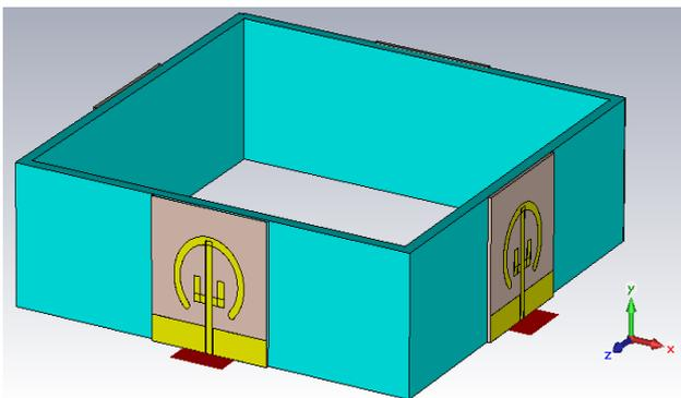
Fig. 2 Proposed array antenna design
