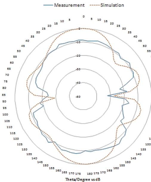
Fig 10. Comparison of simulation and measurement of radiation pattern at phi=90
