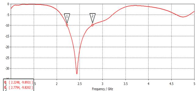
Fig. 4 Reflection coefficient magnitudes (dB) of proposed antenna array
