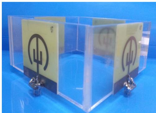
Fig. 6 Fabricated array antenna
