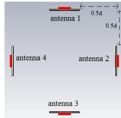
Fig. 3 Array antenna spacing
