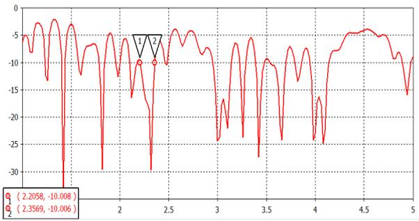
Fig. 9 Measurement result of Reflection coefficient magnitudes (dB) proposed microstrip array antenna
