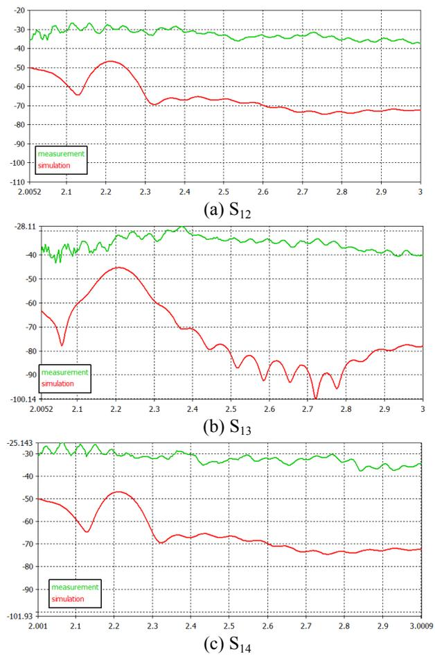
Fig. 7 Mutual Coupling (a)  $S_{12}$  (b)  $S_{13}$  (c)  $S_{14}$  of the array antenna
