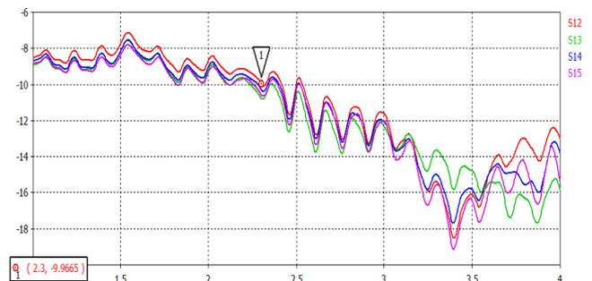
Fig. 8 Insertion loss of splitter COM SP-TX-4B
