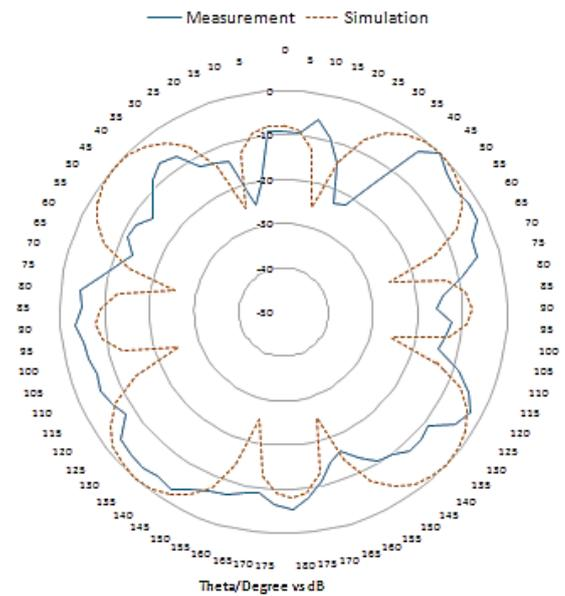
Fig 11. Comparison of simulation and measurement of radiation pattern at phi=0
