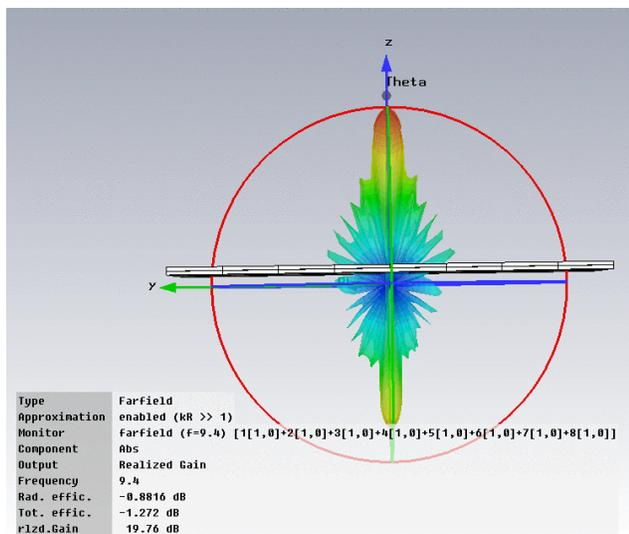
Fig. 3. 3D radiation pattern simulation result of 4 x 8 elements
