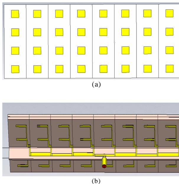
Fig. 1. Antenna design 4 x 8 elements (a) top view first substrate (b) 3D bottom view second substrate
