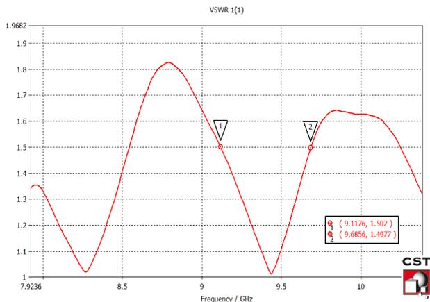
Fig. 2. Simulation result of VSWR 4 x 8 elements
