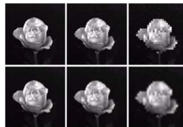
FIGURE 2.23 Top row: images resampled from 128 \times 128 , 64 \times 64 , and 32 \times 32 pixels to 1024 \times 1024 pixels, using nearest neighbor gray-level interpolation. Bottom row: same sequence, but using bilinear interpolation.
