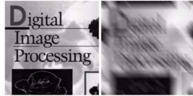
(a) Original image; (b) Result of blurring using function H(u, v) = \frac{T}{\pi(mu + vb)} \sin[\pi(mu + vb)] e^{-j\pi u v} , ( a=b=0.1 and T=1 )
