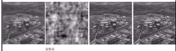
Left: Severe turbulenced image Right: (a) Result of full inverse filtering; (b) Radially limited inverse filter result; (c) Wiener filter result
