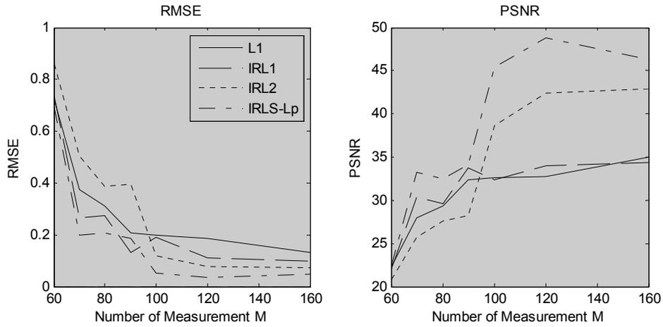
Fig. 3. The RMSE and PSNR value of the approximated scenes using L1, IRL1,IRL2 IRLS-Lp algorithms in different number of measurement M
