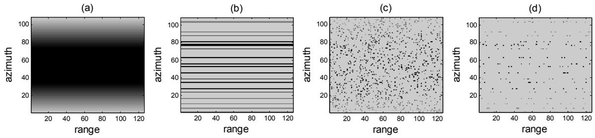
Fig. 1 Compressed SAR signal sampling of target scene (a) full sampling of raw echoes (b) random sampling in slow time (c) random sampling in fast time (d) random sampling in fast time and slow time direction
