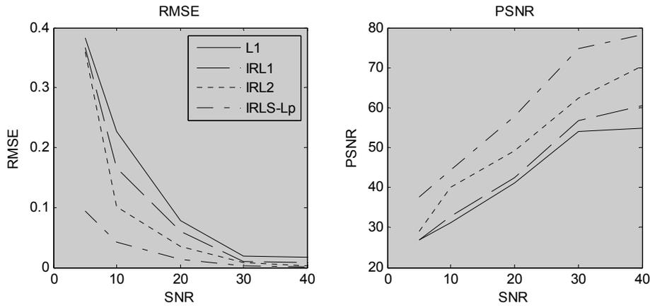
Fig. 4. The RMSE and PSNR value of the approximated scenes using L1, IRL1,IRL2 IRLS-Lp algorithms in different noise level
