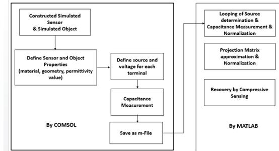
Figure 3. Simulation Set Up for ECVT Imaging
