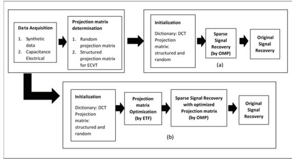
Figure 2. Block Diagram of Simulation Set Up
