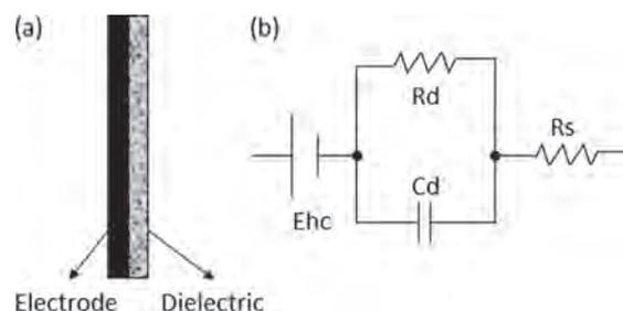
**Figure 1.** (a) Biopotential electrode; (b) equivalent circuit for biopotential electrode.
