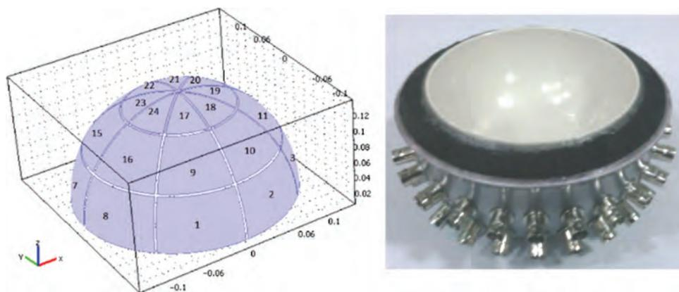
**Figure 5.** A hemisphere 3D sensor 24 channel: Design with unit dimensions in meter (left), physical construction with shielding case and ports (right).
