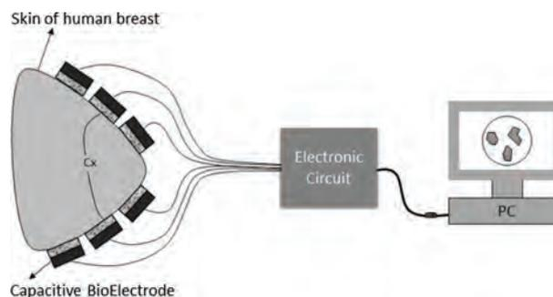
**Figure 2.** Block diagram of breast tissue measurement.
