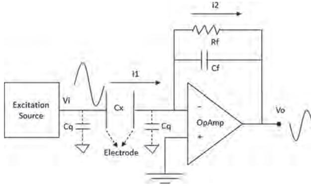
**Figure 3.** Basic of C-V circuit.
