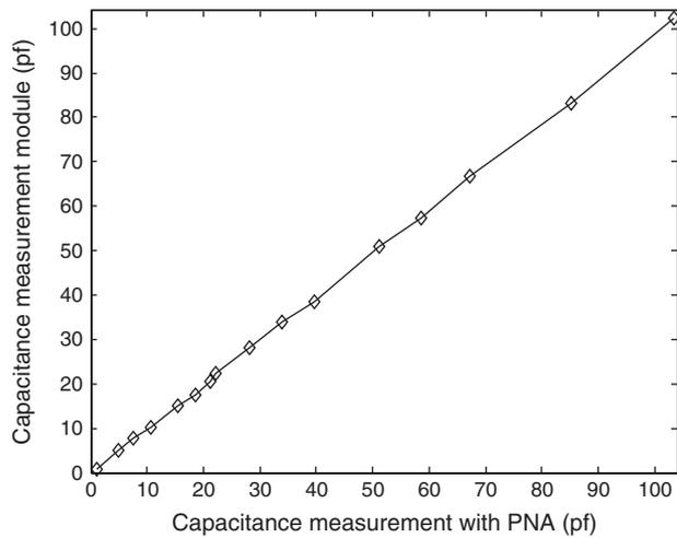
**Figure 6.** Comparison of measurement capacitor between system and PNA.
