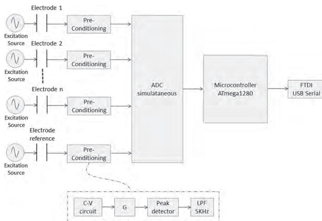
**Figure 4.** Block diagram of signal processing.
