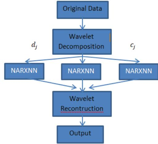
Figure 2. Wind Power Forecast Model with WD-NN
