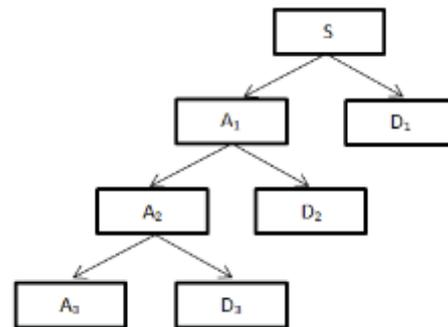
**Figure 1. Decomposition structure of the wavelet transformation for level 3**
