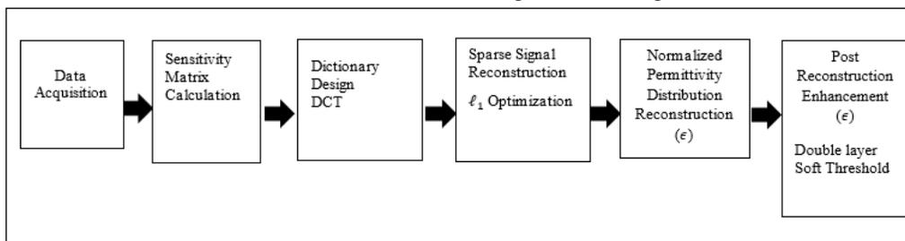
Fig 2. Enriched Compressive Sensing Based Method for ECVT Static Imaging
