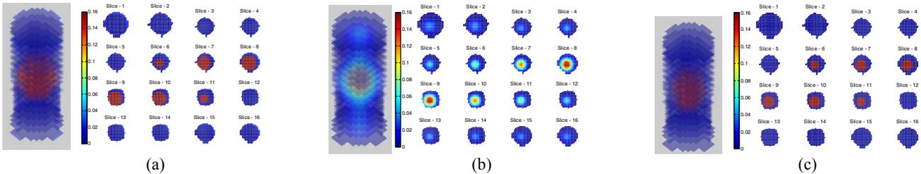
Fig 8. ECVT Static Imaging on High Dielectric Contrast (1:70)
