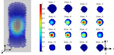
Fig 6. The ECVT Imaging By CS-l1-Hard Threshold (CD:1:6)
