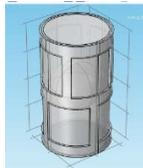
Fig 3. Cylindrical Sensor with 8 electrodes,  $d=10$  cm,  $h=20$  cm, Source [12] CTech Lab
