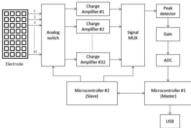
Fig. 6. Block diagram of measuring method for each DAS
