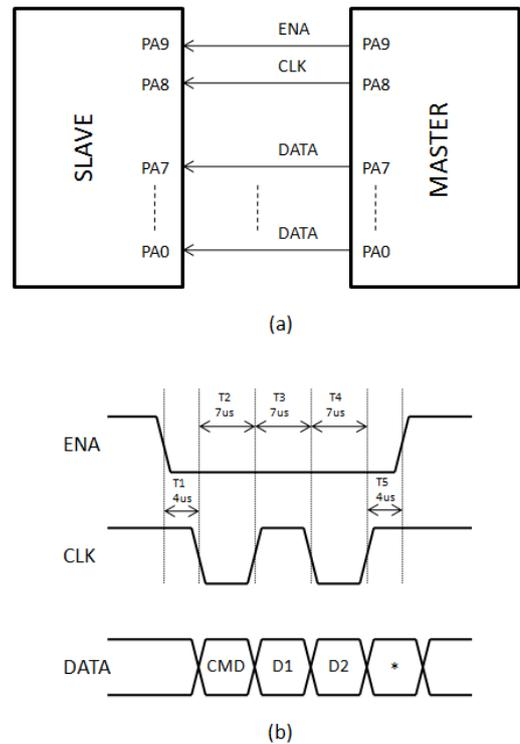
Fig. 7. Protocol communication between Master and Slave microcontrollers; (a) Block diagram; (b) Timing diagram of signal control
