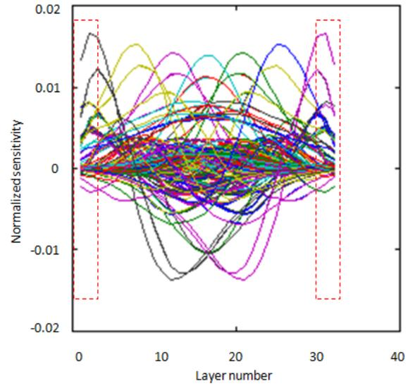
Fig. 3. Axial distribution of normalized sensitivity for all electrode pairs (the dead zones are indicated by the dashed line).
