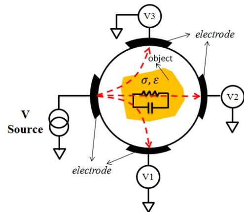
Fig. 1. Principle of capacitance tomography
