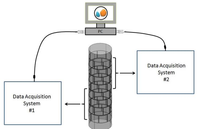
Fig. 4. Block diagram of ECVT Data Acquisition System
