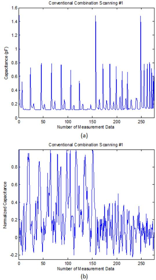
Fig. 9. Signals measurement for first 24 electrodes scanning; (a) Capacitance signal; (b) Normalized capacitance
