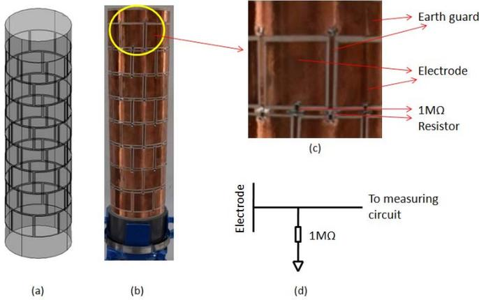
Fig. 2. Proposed capacitive sensor; (a) 8×8 sensor design (b) photograph of the sensor; (c) connection of electrodes in detail; (d) circuit diagram of each electrode
