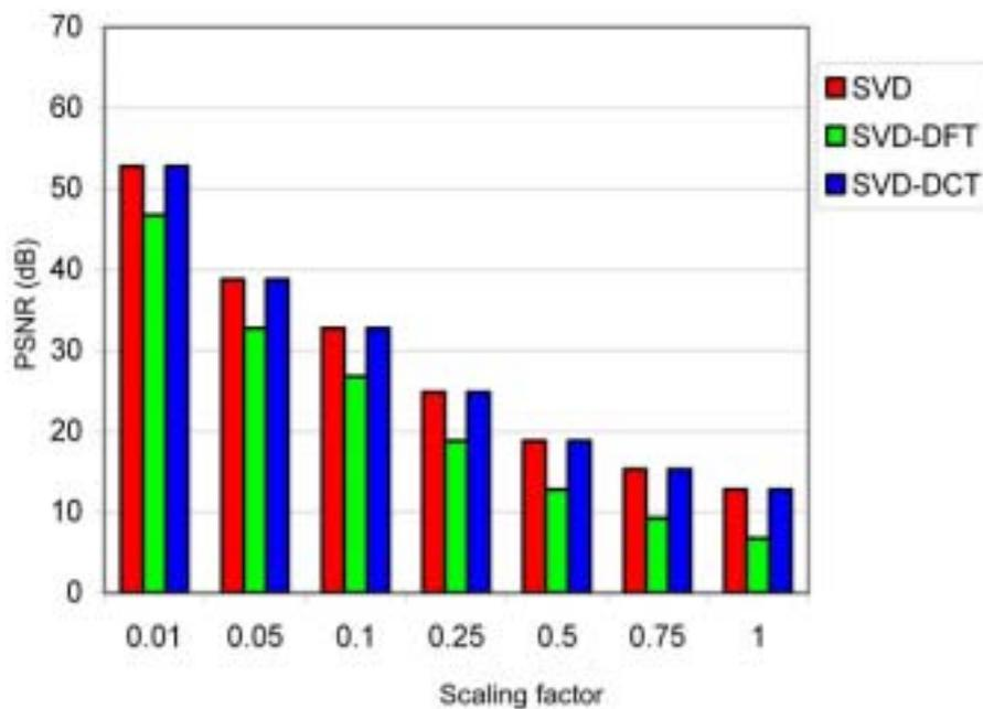
Figure 8. The robustness of each watermarking method to scaling factors.
