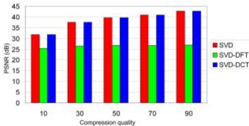
Figure 13. The robustness of each watermarking method to JPEG compression
