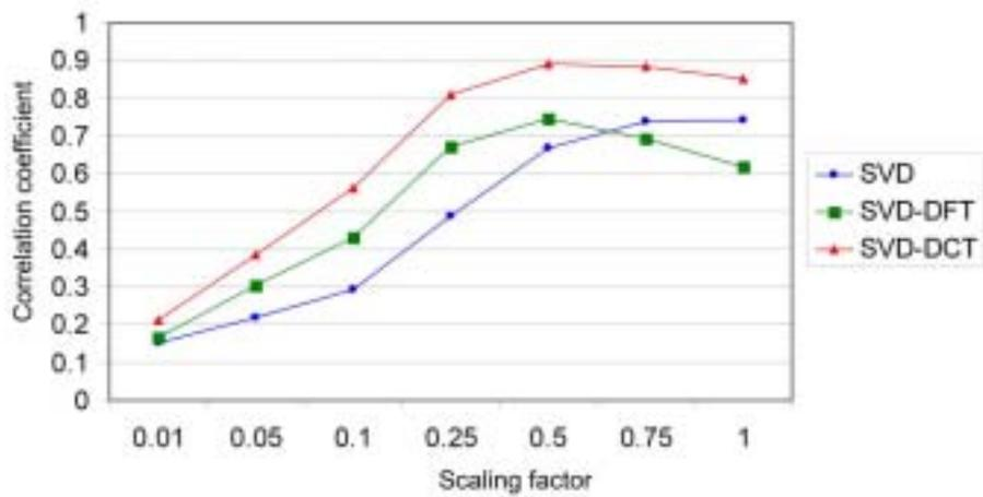
Figure 10. The robustness of each watermarking method to Gaussian noise shown by the correlation coefficient
