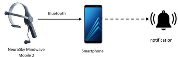
Fig. 2. The block diagram of the hardware system
