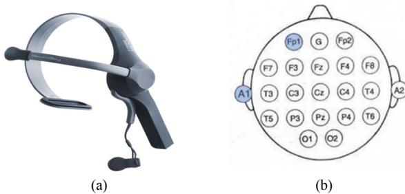
Fig. 1. Single channel EEG a) Neurosky Mindwave 2 BCI device and b) Fp1 electrode's position in 10-20 System
