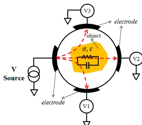
Fig 1. Principle of capacitance tomography
