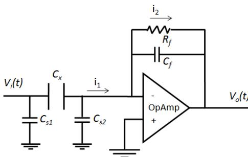
Fig 3. Charge amplifier circuit
