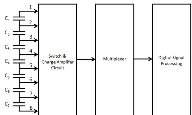
Fig 2. Design of equipment test using dummy capacitor array
