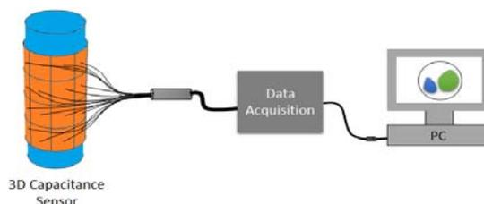
Figure 1. Block diagram of ECVT system
