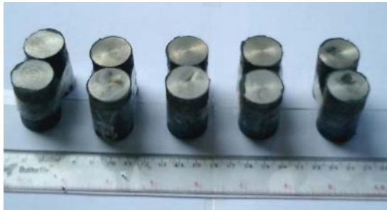
Figure 4: Fracture surfaces of unprepared samples after adhesion test. The shiny surfaces of the substrate show complete WC-Co coating peel off.
