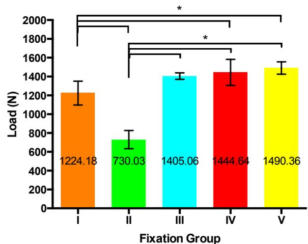
**Figure 5.** Comparison of load to failure upon axial forces among fixation groups. Data are presented as mean  $\pm$  SD.  $n = 4$  /group,  $*p < 0.05$
