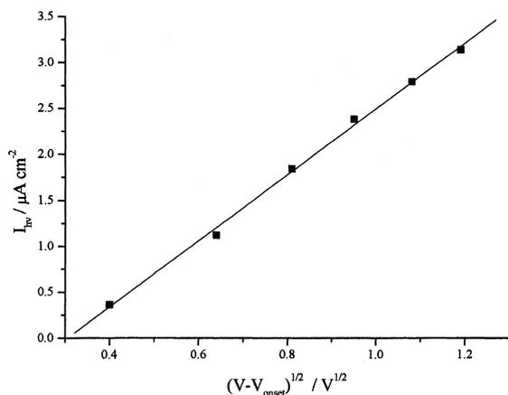
Fig. 5. Plot of photocurrent current density as a function of square root of applied potential on the thermal film TiO<sub>2</sub> electrode.
