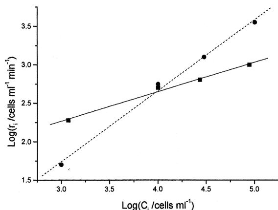
Fig. 10. Plot of  $\log$  initial rate of reaction at sol-gel (—) and thermal film (- - -) electrodes against  $\log$  initial concentrations of *E. coli* in the range  $1 \times 10^3$  to  $1 \times 10^5$  cells ml<sup>-1</sup>. Electrolysis performed under potentiostatic control (1.0 V vs Ag/AgCl).
