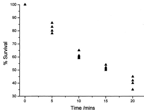
Fig. 6. A typical disinfection profile of *E. coli* ( $1 \times 10^4$  cells ml<sup>-1</sup>) at a thermal film electrode. Potential held at 1.0 V vs Ag/AgCl (LIGHTON).
