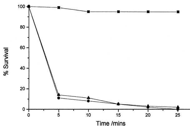
Fig. 8. Effect of applied potential on rate of disinfection of *E. coli* bacteria in tap water ( $1 \times 10^3$  cells ml<sup>-1</sup>) at a TiO<sub>2</sub> sol-gel electrode. Potentials vs Ag/AgCl. Experimental conditions: (■) light off at 1.0 V, (▲) light on at 0.5 V and (●) light on at 1.0 V.
