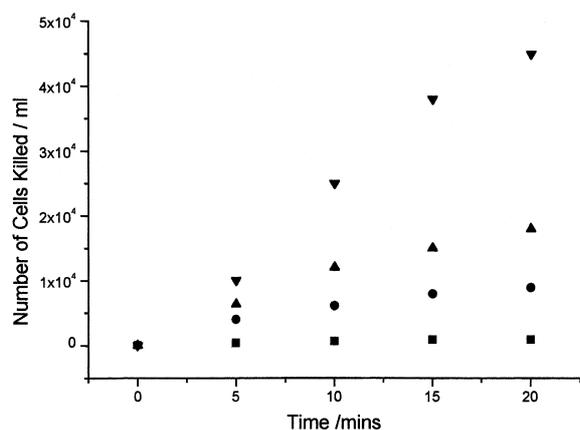
Fig. 9. Number of cells killed per millilitre of sample against time at a TiO<sub>2</sub> thermal film. Initial cell concentrations expressed as cells ml<sup>-1</sup>: (■)  $1 \times 10^3$ , (●)  $1 \times 10^4$ , (▲)  $3 \times 10^4$  and (▼)  $1 \times 10^5$ .
