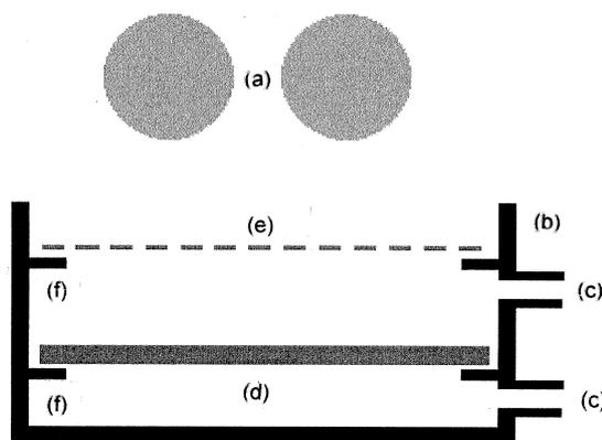
Fig. 2. Schematic representation of the photoelectrochemical reactor. (a) 2 × 8 W UVA lamps; (b) Pyrex glass cell; (c) inlet/outlet ports; (d) 5 cm × 5 cm × 0.2 cm TiO<sub>2</sub> electrode; (e) Ni mesh counter electrode; (f) glass supports. The Ag/AgCl reference electrode is omitted for clarity.
