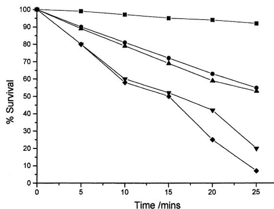
Fig. 7. Effect of applied potential on rate of disinfection of *E. coli* bacteria ( $1 \times 10^4$  cells ml<sup>-1</sup>) at a TiO<sub>2</sub> thermal film. Potentials vs Ag/AgCl. Experimental conditions: (■) light off at open circuit, (+) light off at 1.0 V, (●) light on at 0.1 V, (▲) light on at open circuit, (▼) light on at 0.5 V and (◆) light on at 1.0 V.
