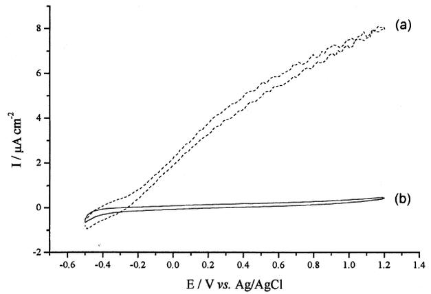
Fig. 3. Cyclic voltammograms of a thermal TiO<sub>2</sub> electrode in tap water (a) u.v. light on. (b) Dark response. Potential vs Ag/AgCl. Scan rate = 100 mV s<sup>-1</sup>.
