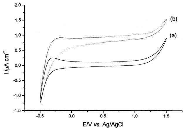
Fig. 4. Cyclic voltammograms of a sol-gel TiO<sub>2</sub> electrode in tap water. (a) Dark response, (b) u.v. light on. Scan rate = 100 mV s<sup>-1</sup>. Potential vs Ag/AgCl.
