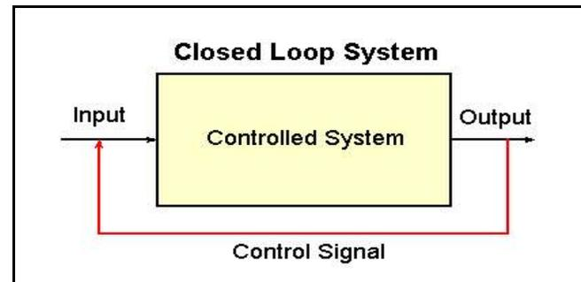
Figure 2-2. A closed loop control system. The controlled system is indicated by the rectangle. Also indicated are the input, output and control signal.
