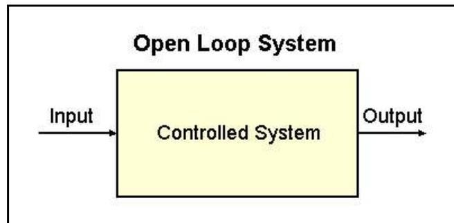
Figure 2-1. An open loop system. The controlled system is indicated by the rectangle. Also indicated are the input to the system and its output.
