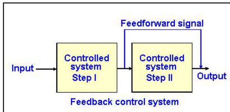
Figure 2-6. Block diagram of a feedforward control system.
