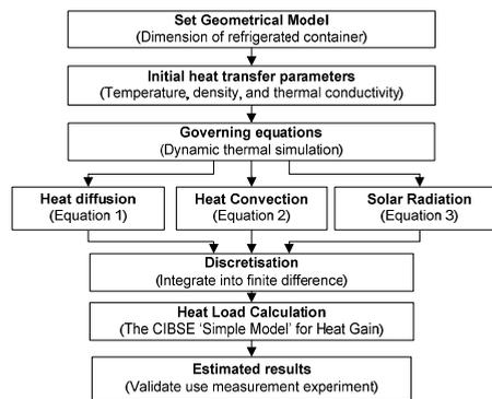
Fig. 1. Calculation process of the simulation study
