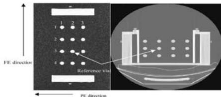
FIG. 7. A CT image (at left) and a sagittal MR image (at right) of the phantom. The directions of the PE and FE, the index for the columns, and rows of the vials are shown.
