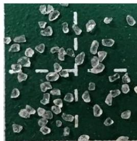
**Figure 1.** PMMA porogen granules with a size of  $300\text{-}500\ \mu\text{m}$ .
